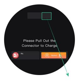
1) These icons mean the EVSE has connected to 4G/Ethernet/Bluetooth/WiFi
