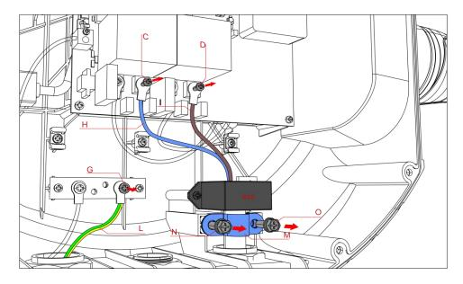
22kW:Unscrew screw C, D, E, F on circuit board and G on copper busbar.
